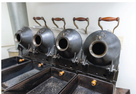
Beans selected for testing go through a small-sample roaster before evaluation.
